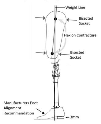
**Note:** The 1315S/1315T is a mechanical 4 bar knee. 4 bar knees are inherently stable, but care needs to be taken to properly bench align the knee with the prosthesis.
