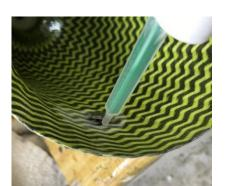
You can locate the Star Nut with a copper rivet that has petroleum jelly on the tip and inserted through the hole and the Star Nut placed onto it.
